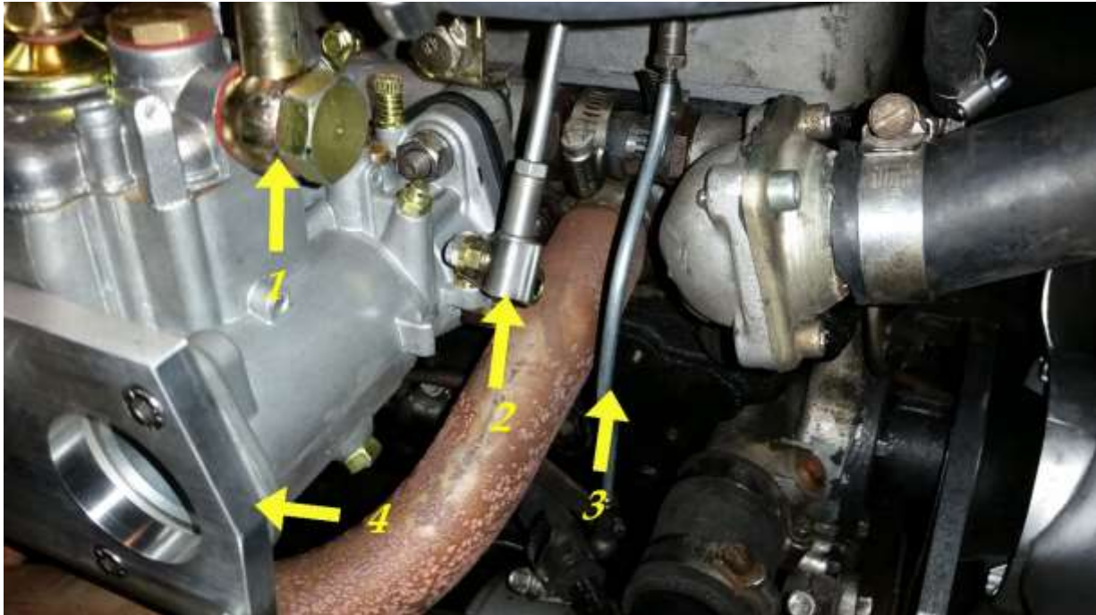
1) Fuel Inlet Banjo 2) Throttle Rod 3) Primary Throttle Rod 4) Plenum Adaptor Plate
