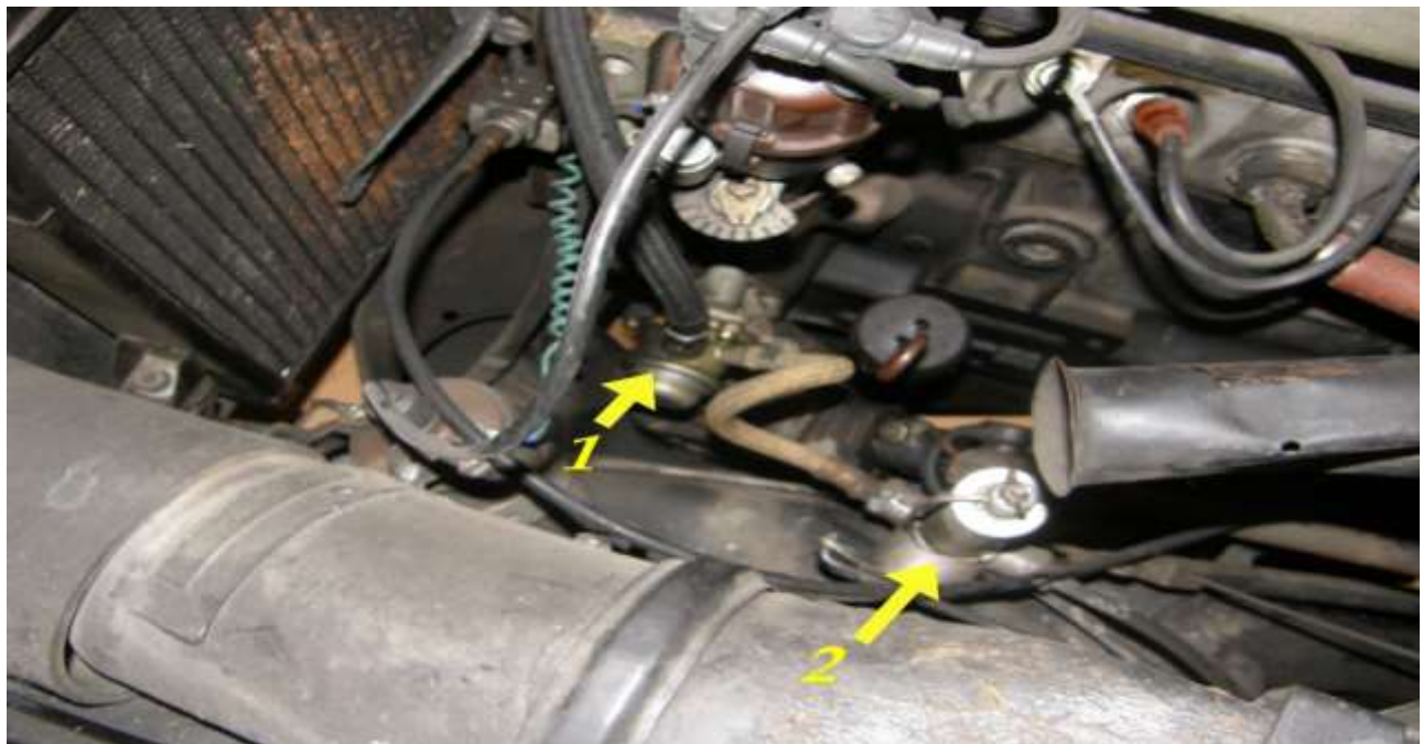
1) Manual Priming Fuel Pump 2) Reserve Fuel Switching Valve/filter
