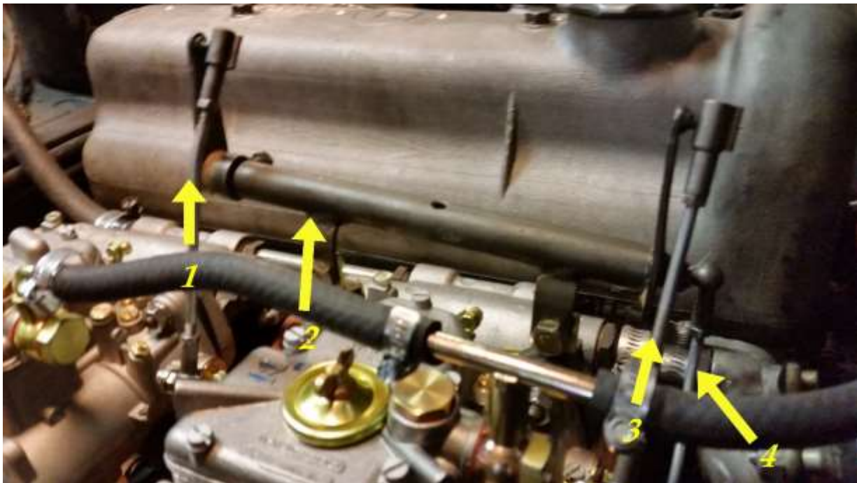
1) Rear Carburetor Throttle Linkage Rod 2) Pivot Arm Assembly 3) Front Carburetor Linkage Rod 4). Primary Throttle Linkage Rod
