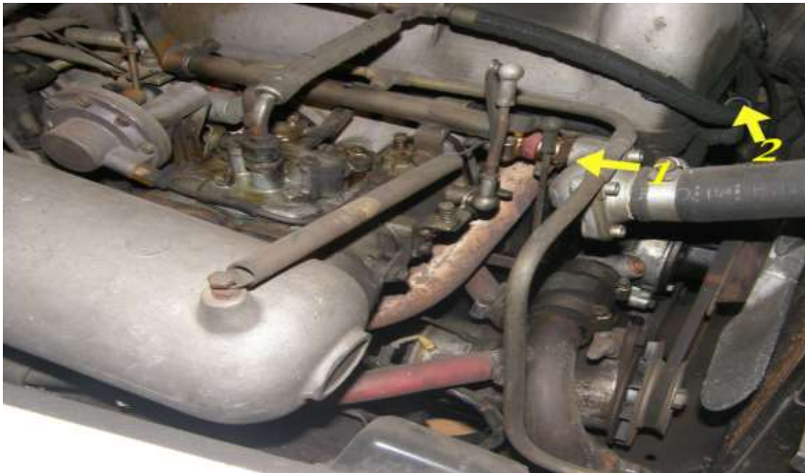
1) Primary, Linkage Rod 2) Metal Fuel Line to Pump
